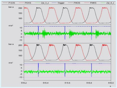
Measurement signals of defect and intact cylinder
